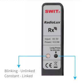
Press the link button on the Tx, to link all Rx in the receiving environment. Long Press the link button, the Tx will unlink to all Rx. You don't need to operate on the Rx as they are hanging on the ceiling.
